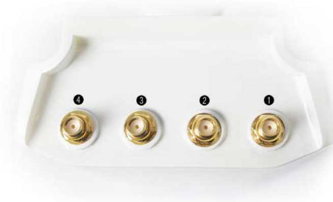
Figure 1.2: Antenna connectors of MX1901/2 Gateway.
